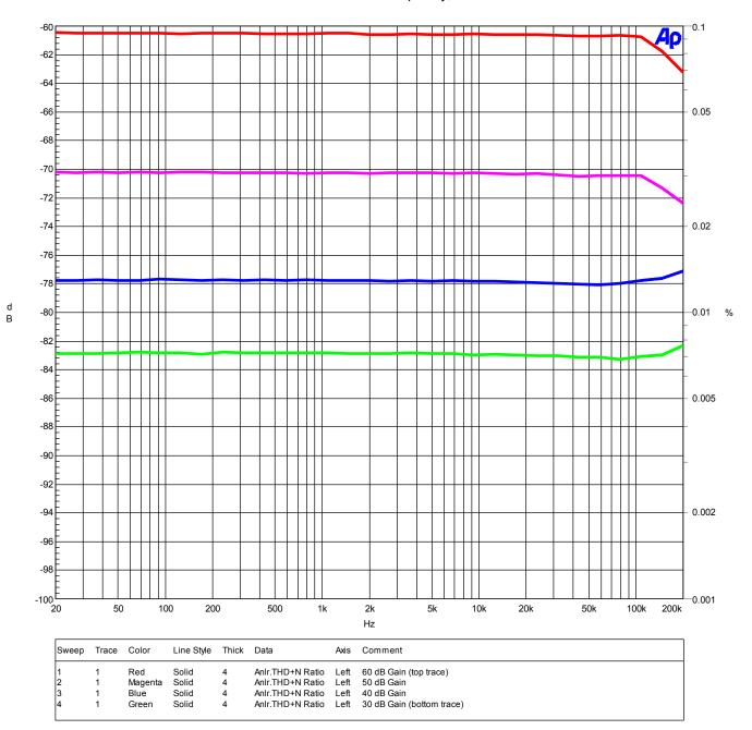
This graph shows that THD+N does not rise above noise – even at very high frequencies. The 500 kHz measurement bandwidth elevates the noise by 28 dB relative to a 20 kHz measurement bandwidth.
