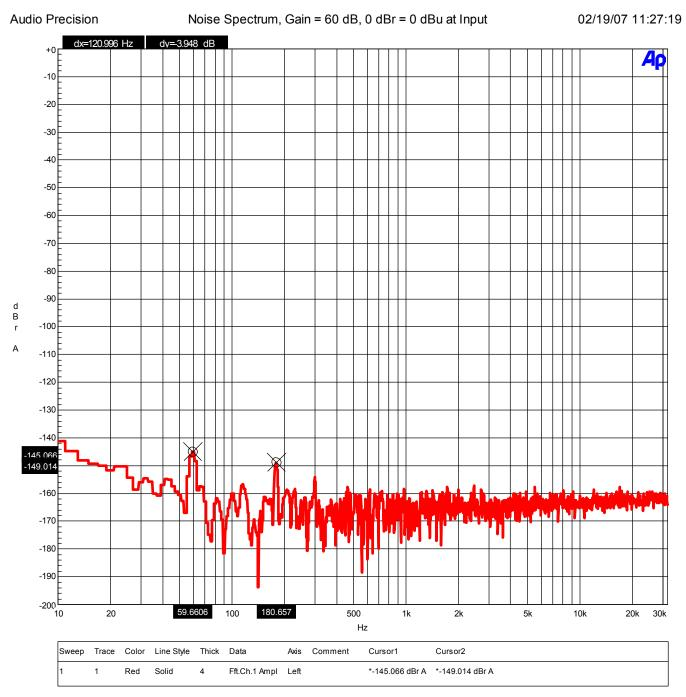
The above graph demonstrates that the **PRE420** is free of hum and noise. The highest tone is 60-Hz line-related hum and is at a level equivalent to an input level of -145 dBu. 180-Hz hum is at an equivalent input level of -149 dBu.
