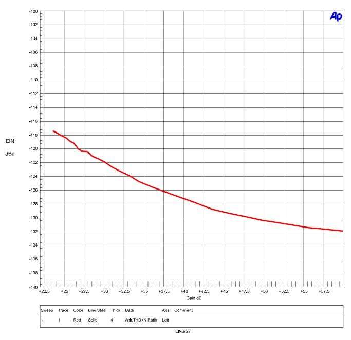
The above plot shows the Equivalent Input Noise (EIN) of the **PRE420** as a function of gain. Measurement bandwidth is 20 Hz to 20 kHz. Input termination is 150 Ohms.
