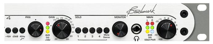
The **PRE420** is a 4-channel microphone preamplifier/mixer and is designed to achieve the highest performance available in a microphone preamplifier. The **PRE420** is designed for maximum transparency, wide bandwidth, low-noise, low-distortion, and superior RF immunity. It is well suited for the most demanding applications in studios and live venues.
