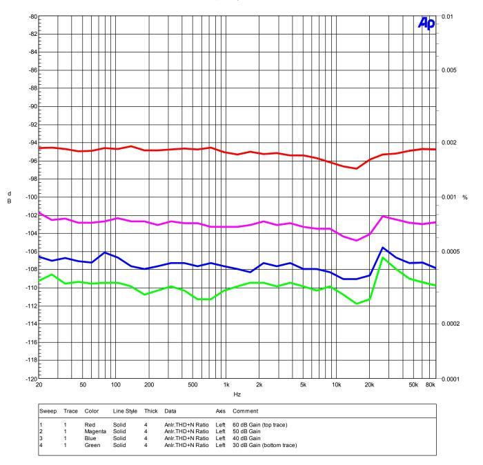
This graph shows that THD+N does not rise with frequency – even at maximum gain.
