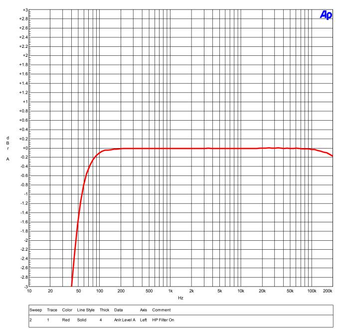
The above graph shows the response of the 40 Hz high-pass filter. Response is -3 dB at 40 Hz with a slope of 12 dB/octave.
