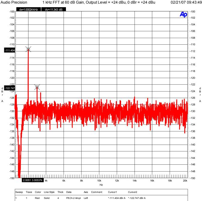
The above FFT plot shows that the **PRE420** has very little harmonic distortion. The 1 kHz test tone is notched out with a THD analyzer to improve the resolution of the test. Distortion is exceptionally low. 2<sup>nd</sup>-harmonic distortion measures better than -111 dB. 3<sup>rd</sup>-harmonic distortion measures better than -122 dB. Note the absence of higher-order harmonics.
