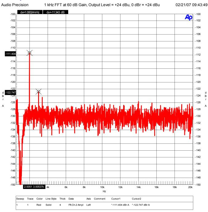
The above FFT plot shows that the PRE420 has very little harmonic distortion. The 1 kHz test tone is notched out with a THD analyzer to improve the resolution of the test. Distortion is exceptionally low.  $2^{nd}$ -harmonic distortion measures better than -111 dB.  $3^{rd}$ -harmonic distortion measures better than -122 dB. Note the absence of higher-order harmonics.
