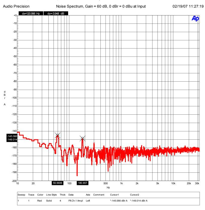
The above graph demonstrates that the PRE420 is free of hum and noise. The highest tone is 60-Hz line-related hum and is at a level equivalent to an input level of -145 dBu. 180-Hz hum is at an equivalent input level of -149 dBu.
