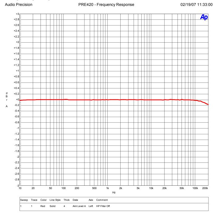
The above graph shows the frequency response of the PRE420 with the 40 Hz high-pass filter off. The amplitude response measures -0.020 dB at 10 Hz and -0.165 dB at 200 kHz. The bass response extends well below the 10-Hz limitation of the test equipment, and the high-frequency response extends well above the 200 kHz limit of the test equipment.
