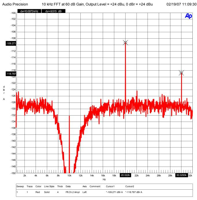
The above FFT plot shows that the PRE420 has very little harmonic distortion at high frequencies. The 10 kHz test tone is notched out with a THD analyzer to improve the resolution of the test. The  $20\text{-kHz}~2^{\text{nd}}$ -harmonic distortion measures better than -109 dB. The  $30\text{-kHz}~3^{\text{rd}}$ -harmonic distortion measures better than -118 dB.
