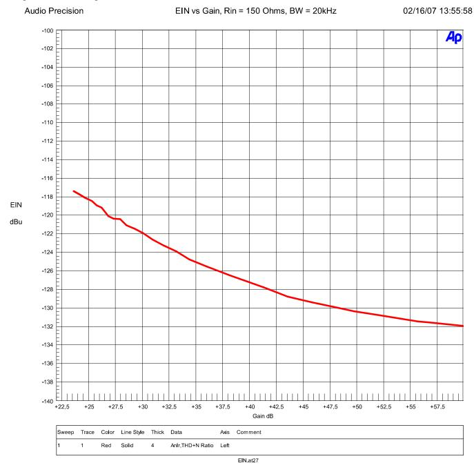
The above plot shows the Equivalent Input Noise (EIN) of the PRE420 as a function of gain. Measurement bandwidth is 20 Hz to 20 kHz. Input termination is 150 Ohms.
