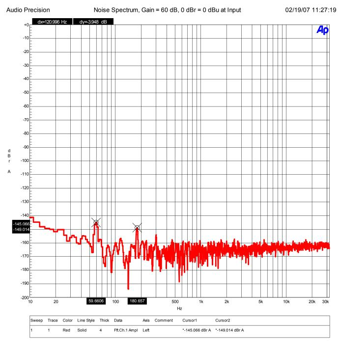
The above graph demonstrates that the MPA1 is free of hum and noise. The highest tone is 60-Hz line-related hum and is at a level equivalent to an input level of -145 dBu. 180-Hz hum is at an equivalent input level of -149 dBu.
