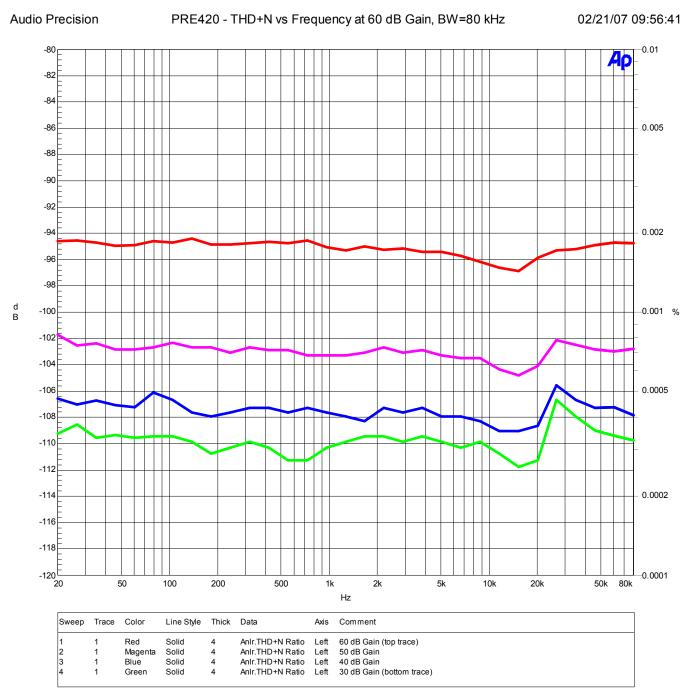
This graph shows that THD+N does not rise with frequency – even at maximum gain.
