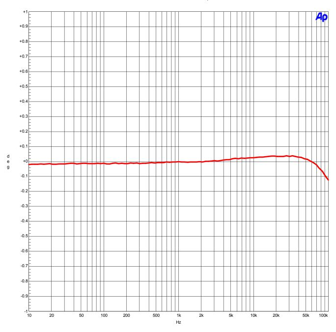
This graph shows that the differential phase is significantly better than  $\pm$  0.05 degrees from 10 Hz to 20 kHz.
