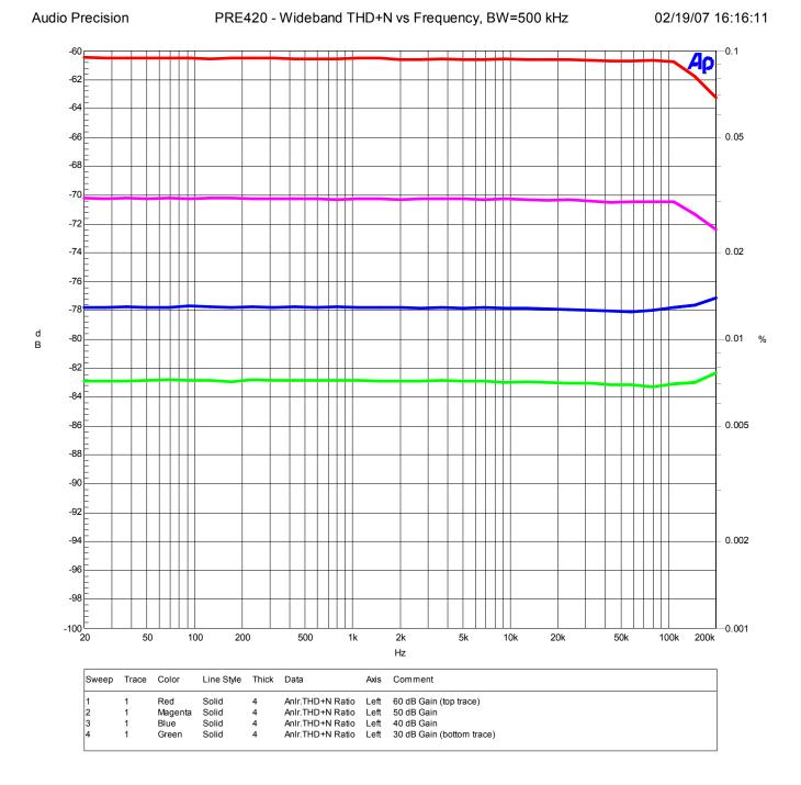
This graph shows that THD+N does not rise above noise – even at very high frequencies. The 500 kHz measurement bandwidth elevates the noise by 28 dB relative to a 20 kHz measurement bandwidth.
