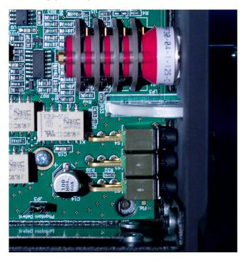
CAUTION: ALWAYS DISCONNECT POWER FROM THE MPA1 FOR FIVE MINUTES BEFORE ADJUSTING THE PHANTOM DEFEAT JUMPER.
