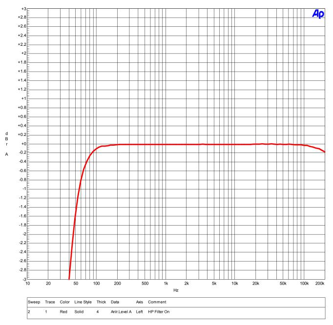
The above graph shows the response of the 40 Hz high-pass filter. Response is -3 dB at 40 Hz with a slope of 12 dB/octave.
