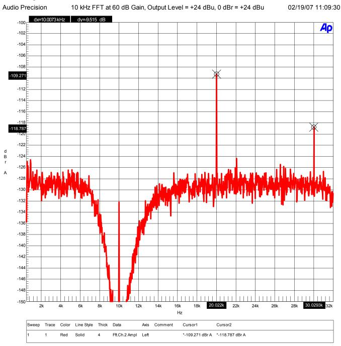
The above FFT plot shows that the MPA1 has very little harmonic distortion at high frequencies. The  $10~\rm kHz$  test tone is notched out with a THD analyzer to improve the resolution of the test. The  $20~\rm kHz$   $2^{\rm nd}$ -harmonic distortion measures better than -109 dB. The  $30~\rm kHz$   $3^{\rm rd}$ -harmonic distortion measures better than -118 dB.
