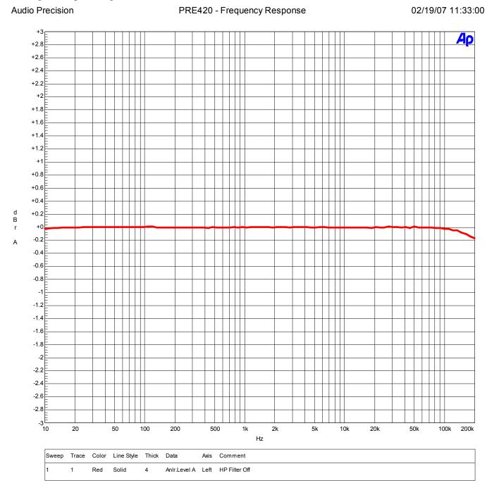
The above graph shows the frequency response of the MPA1 with the 40 Hz high-pass filter off. The amplitude response measures -0.020 dB at 10 Hz and -0.165 dB at 200 kHz. The bass response extends well below the 10-Hz limitation of the test equipment, and the high-frequency response extends well above the 200 kHz limit of the test equipment.
