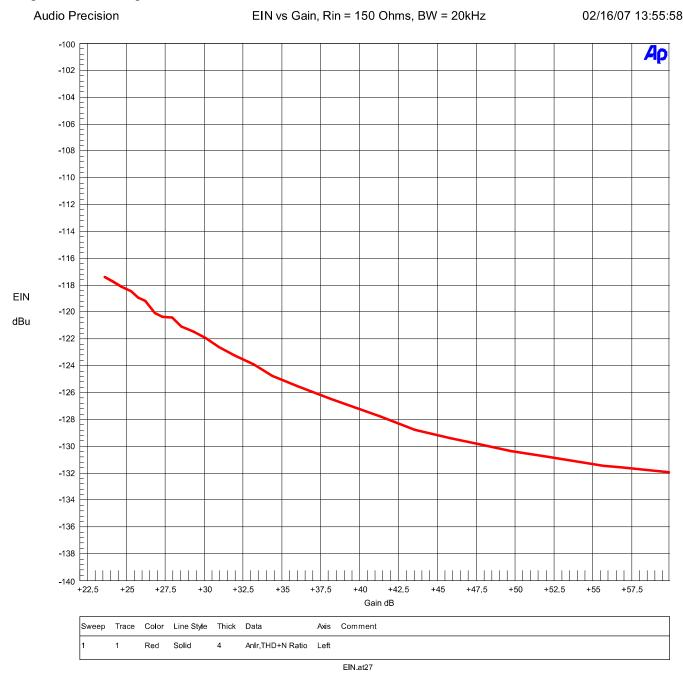
The above plot shows the Equivalent Input Noise (EIN) of the MPA1 as a function of gain. Measurement bandwidth is 20 Hz to 20 kHz. Input termination is 150 Ohms.
