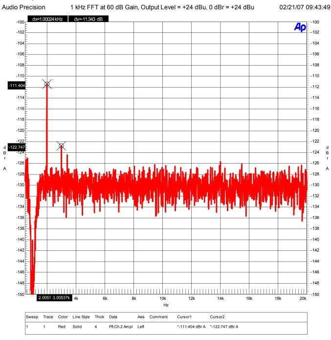
The above FFT plot shows that the MPA1 has very little harmonic distortion. The 1 kHz test tone is notched out with a THD analyzer to improve the resolution of the test. Distortion is exceptionally low.  $2^{nd}$ -harmonic distortion measures better than -111 dB.  $3^{rd}$ -harmonic distortion measures better than -122 dB. Note the absence of higher-order harmonics.
