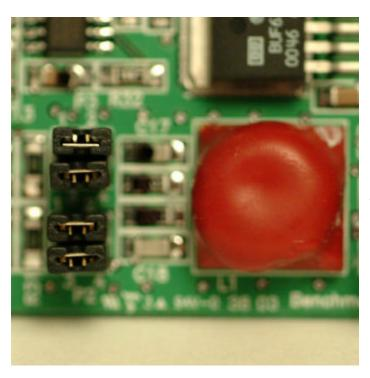
Warning: For Unbalanced Inputs, jumpers must be in this setting to prevent distortion.
