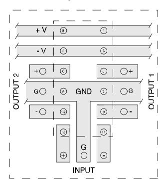
Figure 2.0, LA-1 Connector Pinout
