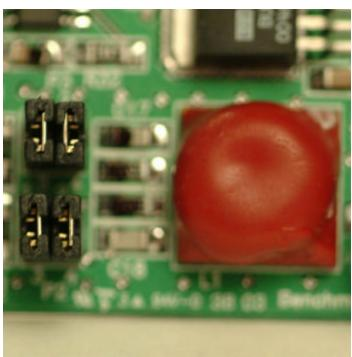
For Balanced Inputs ONLY, select this setting for maximum RF rejection.
