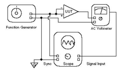
Fig. 2 - Common Mode Rejection Adjustment
