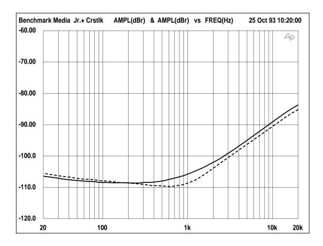
Figure 2. Typical Crosstalk, L into R, and R into L
