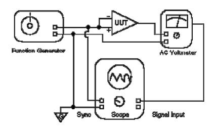
Fig. 2 - Common Mode Rejection Adjustment
