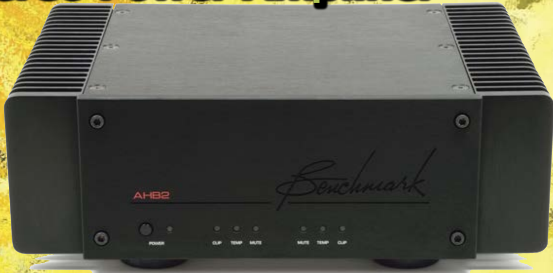
Photo 1: Benchmark's new AHB2 stereo power amplifier uses feed-forward error-correction technology patented by THX that virtually eliminates crossover distortion. The front panel status LEDs indicate Clip, Temperature, and Mute conditions. (Photo courtesy of Benchmark Media Systems, Inc.)
