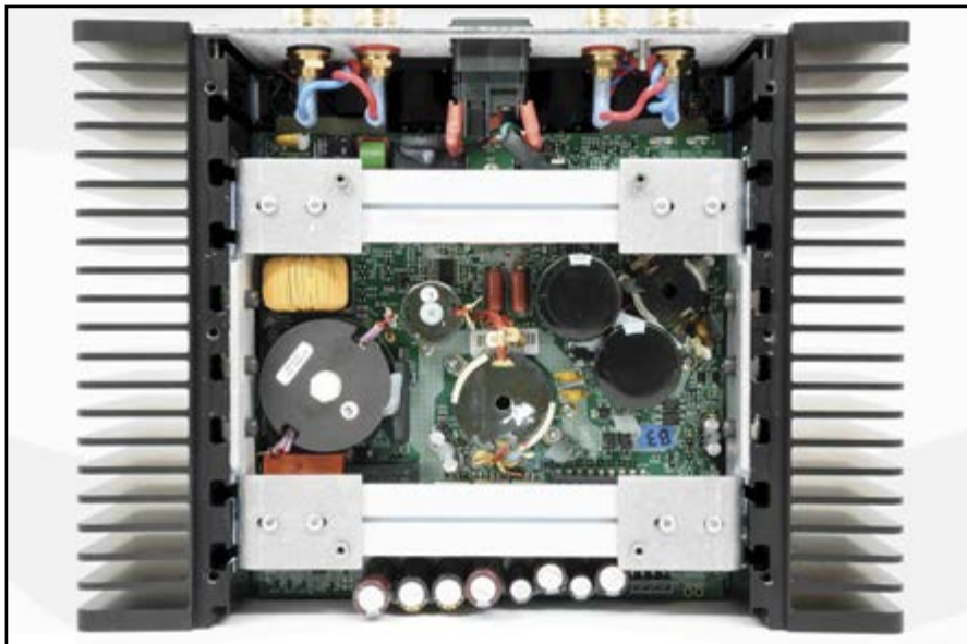
Photo 4: This inside view of the AHB2 shows the top, switching power supply PC board in place. Benchmark's Resonant Switch-Mode supply features lower noise than conventional linear supplies. The high switching frequency allows smaller magnetic components, reducing the strength of stray magnetic fields. (Photo courtesy of Benchmark Media Systems, Inc.)
