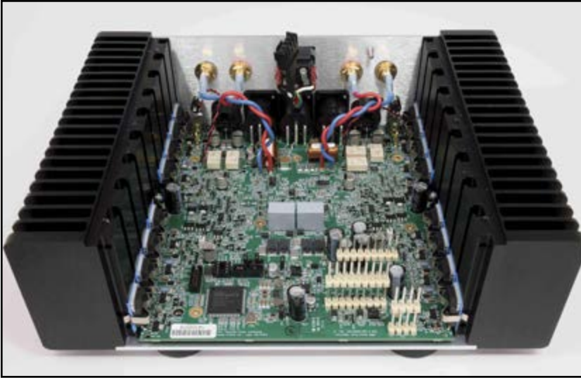
Photo 5: This inside view of the AHB2 shows the lower, main amplifier PC board. The Digital Protection Systems chip is the Xilinx Spartan 6-series FPGA device seen left of center in the front. The bipolar output transistors are mounted to the heatsinks with spring clips to ensure constant pressure regardless of temperature. (Photo courtesy of Benchmark Media Systems, Inc.)
