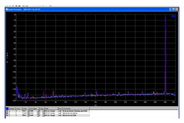
In this graph, there are three measurements of the same 30 kHz digital tone going through the DAC1 USB. The red measurement is the 30 kHz tone coming from the iPad. The cyan measurement is from the Macbook via optical. The blue measurement is from the Macbook via USB. As you can see, they each perform identically, achieving full 96-kHz, 24-bit performance.
