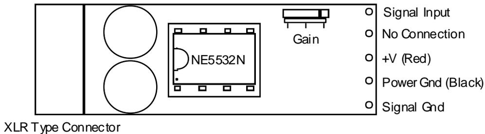
Fig 3.3 DOA-2 Connections and Controls
