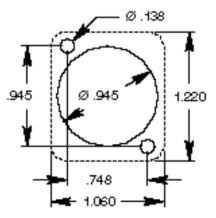
Fig 3.1 Neutrik "D" Series Panel Layout
