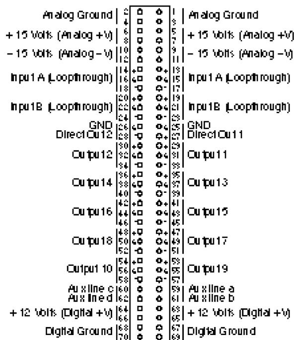
**Figure 3. DA-101 Connector Pinout (View from Rear of Card Frame)**
