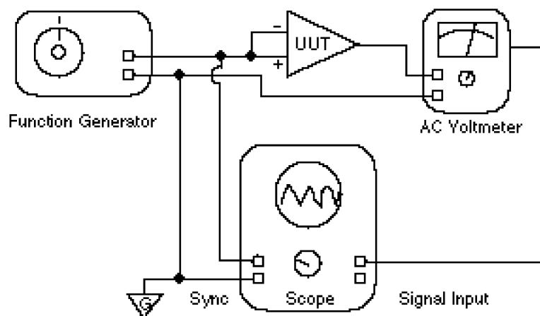
**Fig 4.0 Common Mode Rejection Adjustment**
