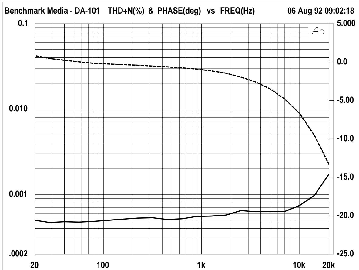
**Figure 1. DA-101 Total Harmonic Distortion and Phase**
