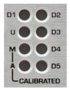
The M and A indicators show that the CALIBRATED mode is active for the MAIN and/or AUX outputs.
