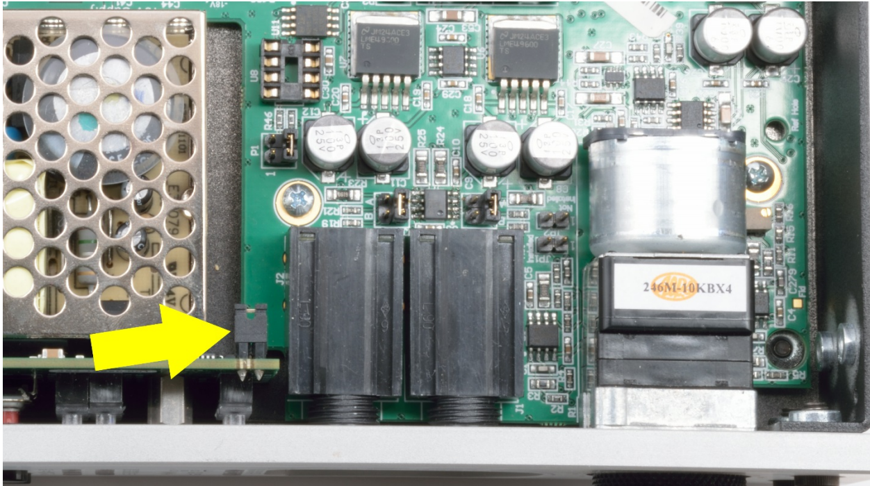
Figure 3 - Add new jumper to the back of the control panel as shown (top two pins of P1).
