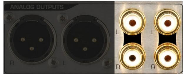
The Left and Right unbalanced outputs use female RCA jacks. The ground connections are bonded to chassis ground at the location where analog ground is bonded to the chassis. This minimizes the effects of ground loops caused by AC currents in the cable shield. The RCA output impedance is very low (30 Ohms). This makes these outputs well suited for driving high-capacitance loads and/or high-capacitance cables.
