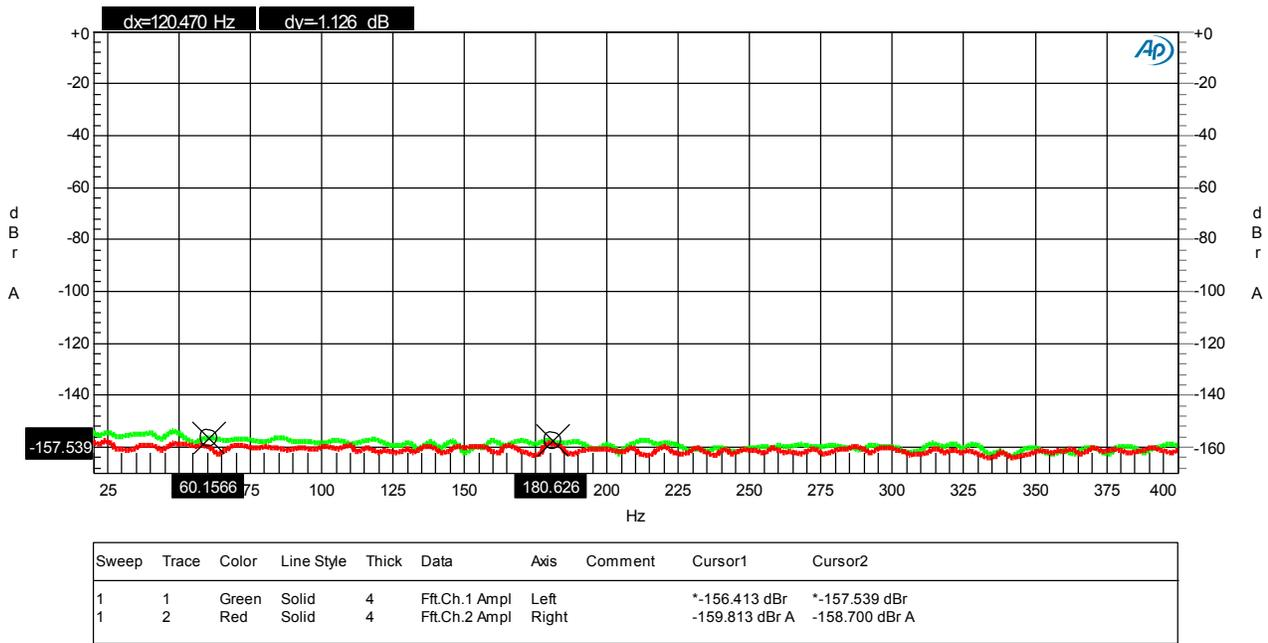
DAC2 - FFT Idle Channel Noise - Low Frequency.at27
