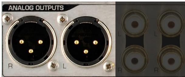
The Left and Right balanced outputs use Neutrik™ gold-pin male XLR jacks. The XLR shell and pin 1 (ground) are both directly bonded to the chassis to prevent currents in the internal ground system. This direct bonding also maximizes RF shielding.
