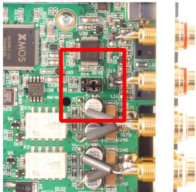
**Figure 8 - Digital PASS-THROUGH Disabled (Factory Default)**
