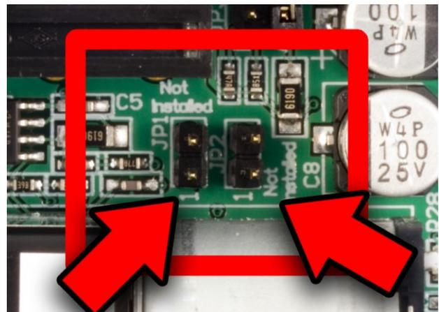
Figure 2 - Headphone Switch Enabled (Factory Default)
