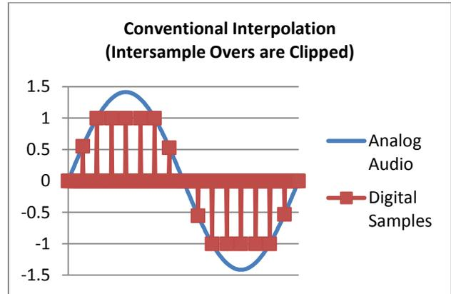
PCM systems can accurately capture peaks that exceed 0 dBFS, but these peaks will overload the oversampling interpolators in most delta-sigma D/A converters. The solution is not to eliminate the interpolation process; the solution is to build interpolators with more headroom.
