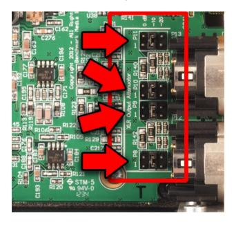
Figure 1 - Attenuators set to -10 dB
