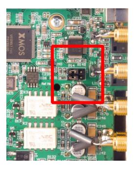
Figure 7 - Digital PASS-THROUGH Enabled
