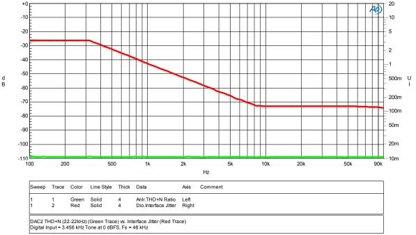
DAC2 - JITTER TOLERANCE.at27
