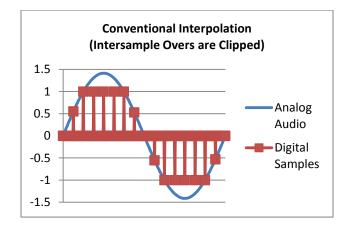
PCM systems can accurately capture peaks that exceed 0 dBFS, but these peaks will overload the oversampling interpolators in most delta-sigma D/A converters. The solution is not to eliminate the interpolation process; the solution is to build interpolators with more headroom.
