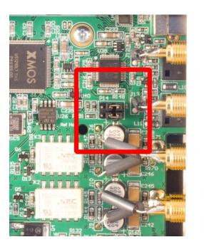
Figure 8 - Digital PASS-THROUGH Disabled (Factory Default)
