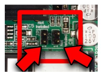
Figure 2 - Headphone Switch Enabled (Factory Default)
