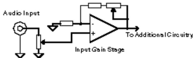
Figure 3 A Common Input Stage
