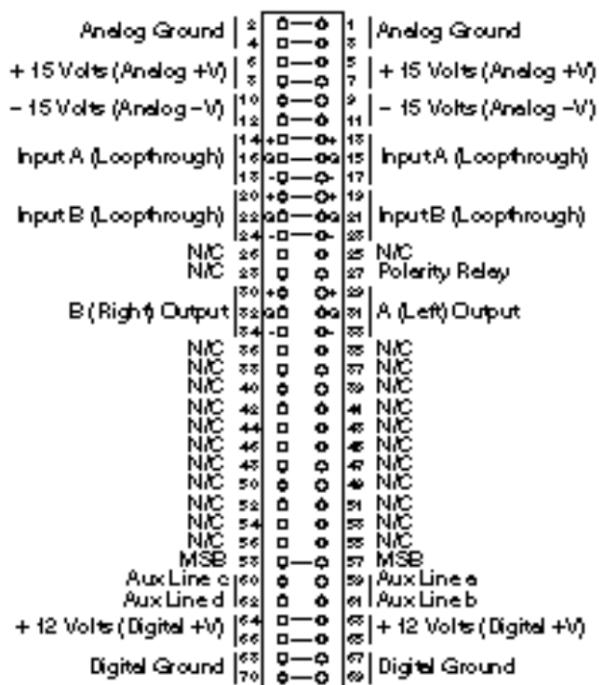
**Fig. 3 - APA-102 SM Connector Pinout (View from Rear of Card Frame)**
