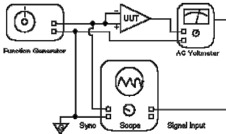
**Fig. 4 - Common Mode Rejection Adjustment**
