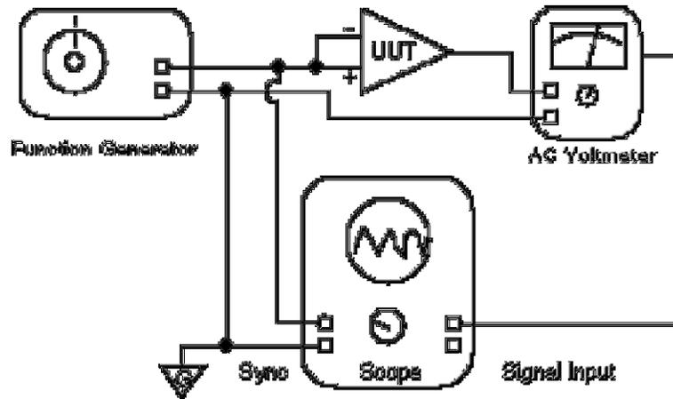
**Fig. 4 - Common Mode Rejection Adjustment**
