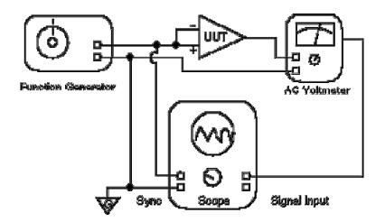
Fig. 4 - Common Mode Rejection Adjustment
