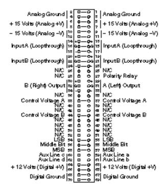
Fig. 3 - APA-102 Connector Pinout (View from Rear of Card Frame)
