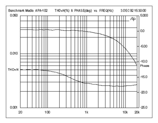
Fig. 1 - Typical APA-102 Total Harmonic Distortion and Phase
