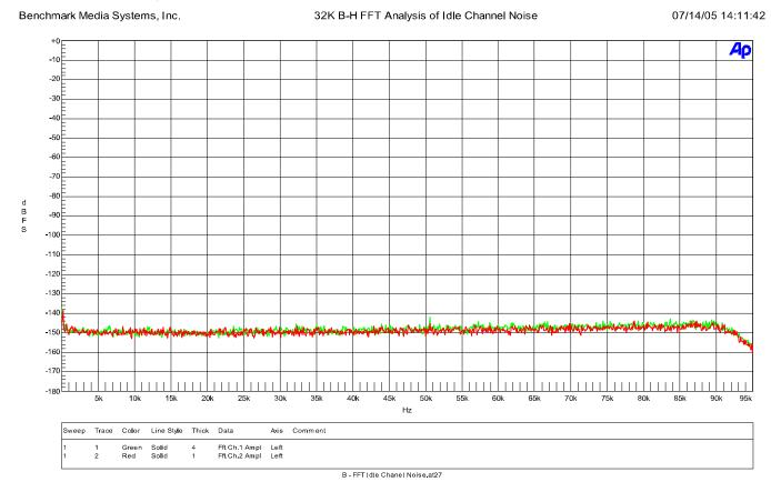
The above graph demonstrates that the ADC1 USB is free from idle tones and clock crosstalk. The highest spurious tone measures -128 dBFS and is AC line related hum. The highest non-line related tone measures -135 dBFS.
