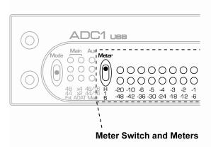
Time constants are built into the meters so all transient peaks can be observed easily. If a transient peak has a duration as short as one digital sample, an LED will be illuminated and remain illuminated long enough to be observed by the human eye.
