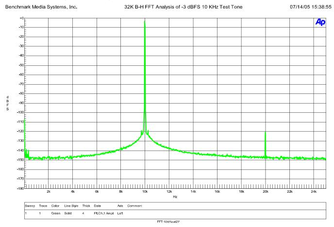
The above FFT plot shows that the ADC1 USB is free from jitter-induced sidebands. Any jitter present at the conversion sampling circuit would produce sidebands equally spaced above and below the 10 kHz test tone. The tone at 20 kHz is due to second harmonic distortion, and measures almost 120 dB below full scale. Note the near absence of spurious tones.
