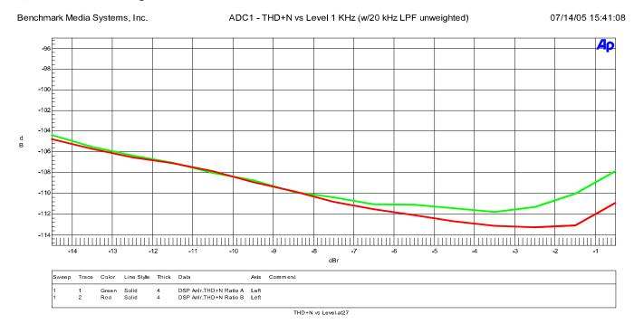
Below -4 dBFS, distortion is lower than the noise floor of the converter. Above -3 dBFS, distortion reaches a maximum value of only -107 dBFS.
