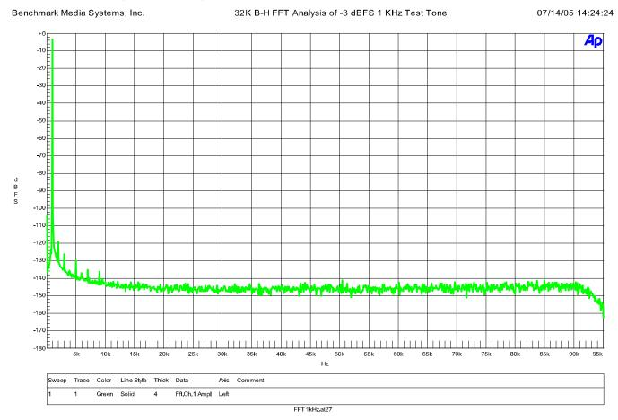
The above FFT plot shows that the ADC1 USB has very little harmonic distortion. Distortion is exceptionally low and is dominated by  $2^{nd}$  harmonic distortion. Note the near absence of spurious tones.
