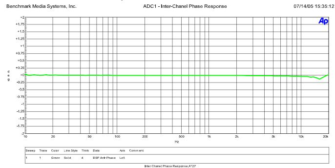
This graph shows that the differential phase is significantly better than  $\pm$  0.25° from 10 Hz to 20 kHz.
