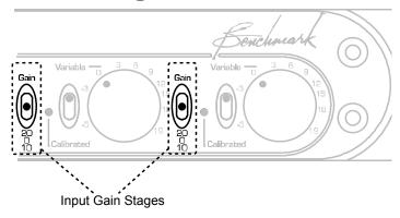
The First-Stage Gain Switches can apply analog gain (0, 10, or 20 dB) to the left and/or right channel. Both channels have their own dedicated switches. The First-Stage Gain can be used in 'Calibrated' or 'Variable' mode.
