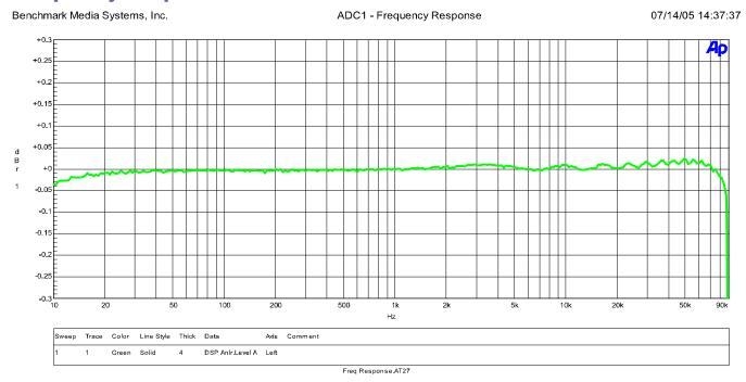
The above graphs show the frequency response of the ADC1 USB when it is operating at a 192-kHz sample rate. Note that the amplitude response is down by less than 0.05 dB at 10 Hz and 80 kHz. The bass response extends well below the 10-Hz limitation of the measurement equipment, and the high-frequency analog response extends well above the 96 kHz bandwidth of 192 kHz digital audio.
