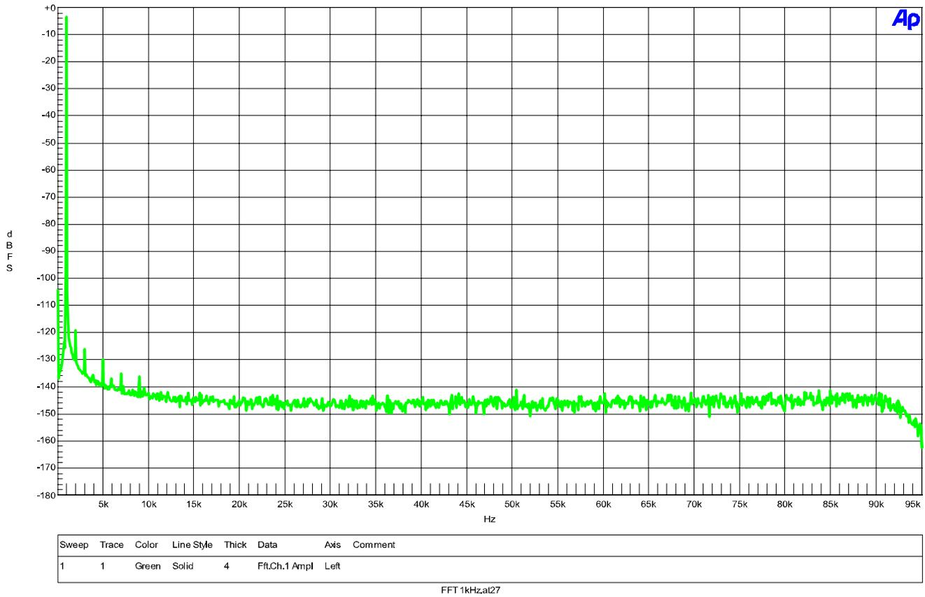
The above FFT plot shows that the ADC1 has very little harmonic distortion. Distortion is exceptionally low and is dominated by 2<sup>nd</sup> harmonic distortion. Note the near absence of spurious tones.
