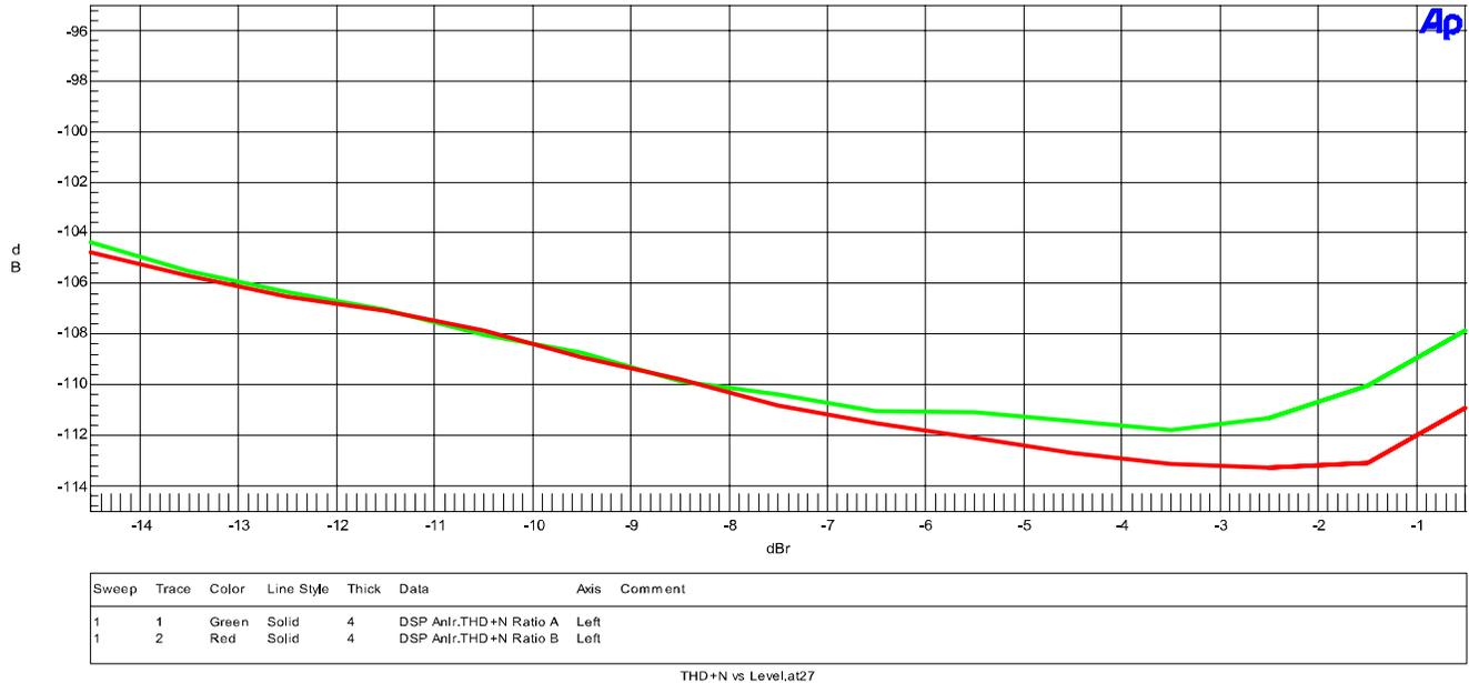
Below -4 dBFS, distortion is lower than the noise floor of the converter. Above -3 dBFS, distortion reaches a maximum value of only -107 dBFS.
