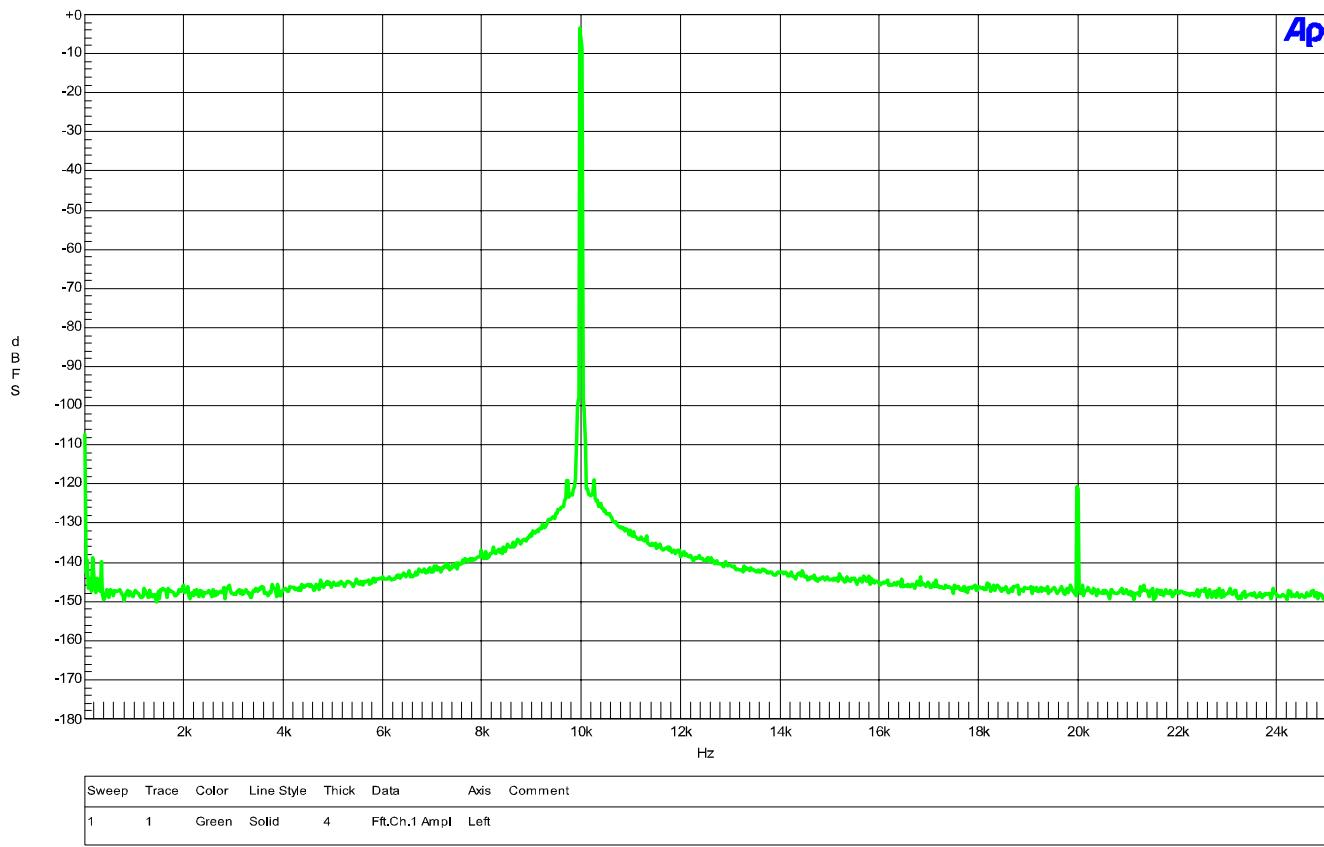
The above FFT plot shows that the ADC1 is free from jitter-induced sidebands. Any jitter present at the conversion sampling circuit would produce sidebands equally spaced above and below the 10 kHz test tone. The tone at 20 kHz is due to second harmonic distortion, and measures almost 120 dB below full scale. Note the near absence of spurious tones.
