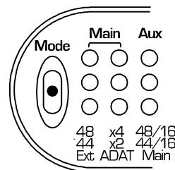
Column one of the display has a "44" LED and a "48" LED. These indicate sample rates of 44.1 kHz and 48 kHz respectively. Column two has an "X2" LED and an "X4" LED. These indicate 2x or 4x multipliers. Multiply the sample rate shown in column one by the multiplier shown in column two. For example, if the 44 and X2 LEDs are on, the sample rate is 88.2 kHz ( $44.1 \times 2 = 88.2$ ).
