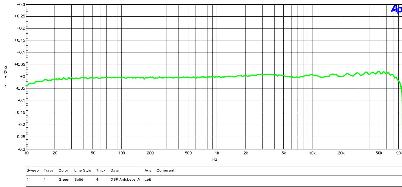
The above graphs show the frequency response of the ADC1 when it is operating at a 192-kHz sample rate. Note that the amplitude response is down by less than 0.05 dB at 10 Hz and 80 kHz. The bass response extends well below the 10-Hz limitation of the measurement equipment, and the high-frequency analog response extends well above the 96 kHz bandwidth of 192 kHz digital audio.
