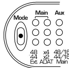
Column one of the display has a "44" LED and a "48" LED. These indicate sample rates of 44.1 kHz and 48 kHz respectively. Column two has an "X2" LED and an "X4" LED. These indicate 2x or 4x multipliers. Multiply the sample rate shown in column one by the multiplier shown in column two. For example, if the 44 and X2 LEDs are on, the sample rate is 88.2 kHz (44.1 x 2 = 88.2).
