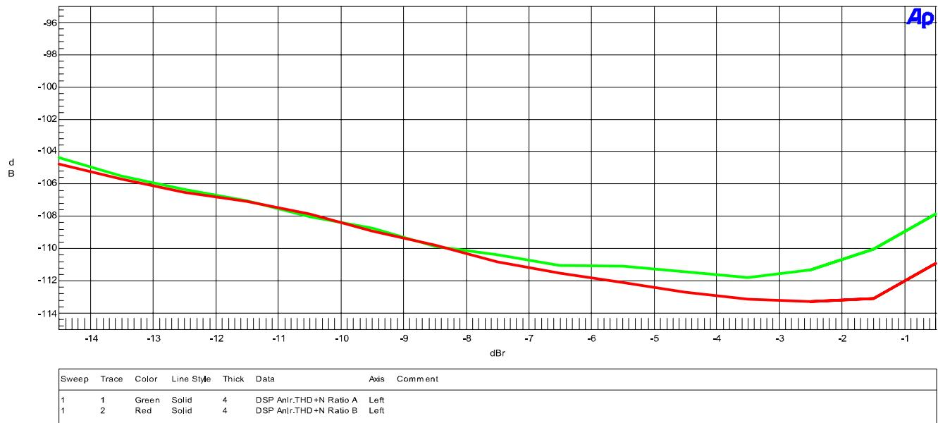
Below -4 dBFS, distortion is lower than the noise floor of the converter. Above -3 dBFS, distortion reaches a maximum value of only -107 dBFS.
