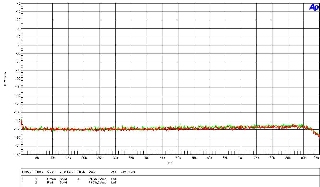
The above graph demonstrates that the ADC1 is free from idle tones and clock crosstalk. The highest spurious tone measures -128 dBFS and is AC line related hum. The highest non-line related tone measures -135 dBFS.
