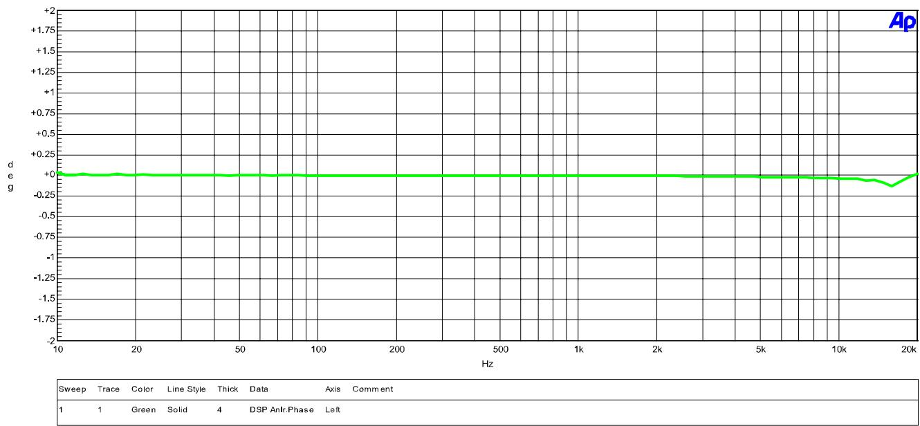
This graph shows that the differential phase is significantly better than  $\pm 0.25^\circ$  from 10 Hz to 20 kHz.
