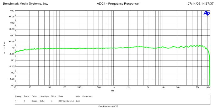
The above graphs show the frequency response of the ADC1 when it is operating at a 192-kHz sample rate. Note that the amplitude response is down by less than 0.05 dB at 10 Hz and 80 kHz. The bass response extends well below the 10-Hz limitation of the measurement equipment, and the high-frequency analog response extends well above the 96 kHz bandwidth of 192 kHz digital audio.
