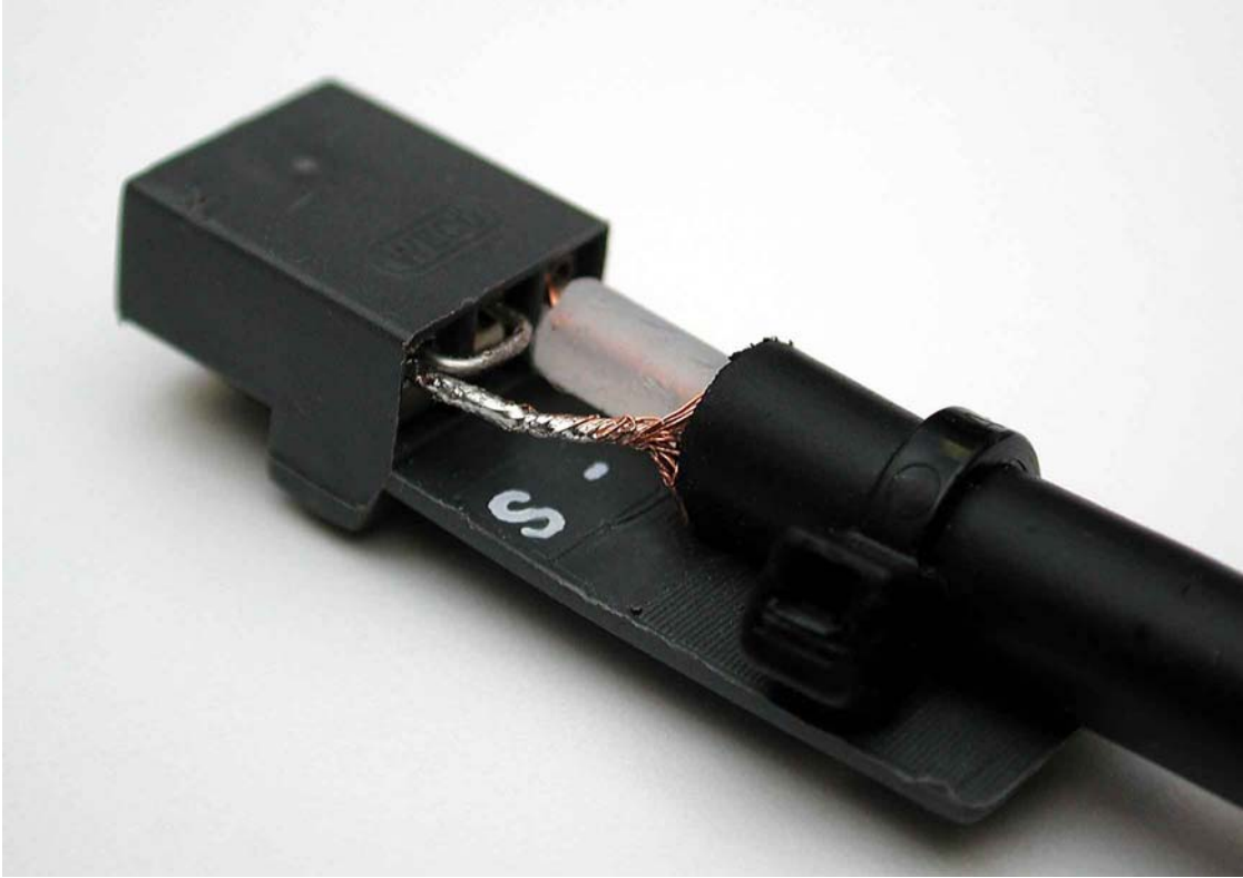
Photo 16 - Coaxial 75-Ohm Unbalanced Digital I/O using WECO HSLConnectors
