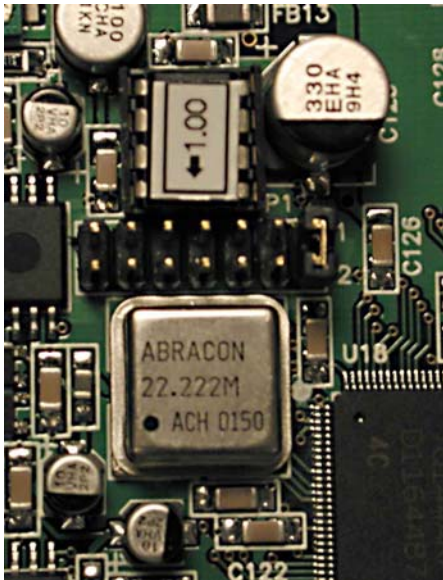
Photo 12 - Fallback Sample-Rate Jumper Locations (shown in default 48 kHz position)
