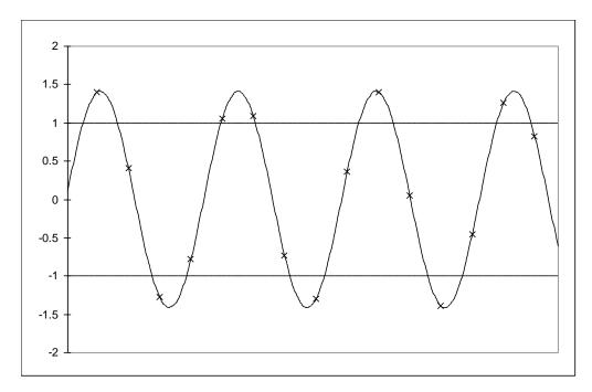
Figure 1 10 kHz Tone at +3 dBFS (1 and -1 represent clip levels)
