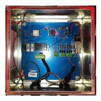
The *Utility Watch* electric utility voltage sensor constantly monitors utility voltage and generates an alarm if the utility power fails.
