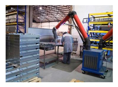
Spark Safe has been developed primarily for the use of operatives welding or undertaking other forms of hot works. Spark Safe is a two part, all rubber constructed anti-fatigue matting with special heat repellent properties to withstand sparks and hot metal fragments
