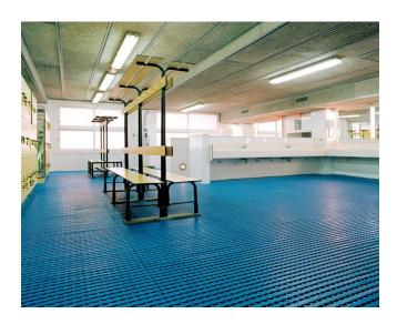
The Herontile system has a simple click joining mechanism designed to cover large floor areas seamlessly and easily. It provides a hygienic, safe and attractive surface with permanent antifungal and anti-bacterial additives.
