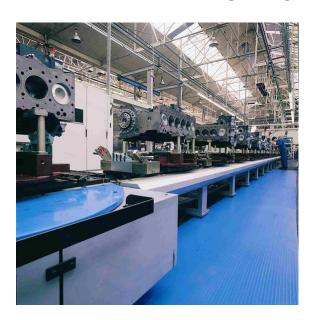
Flexi Tread is a highly durable heavy duty vinyl matting that provides electrical resistance. It insulates from the dangers of electric shock, meeting DIN/EN 60243-1 with a breakdown voltage of 27kv.
