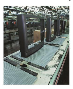
Flexi Ridge is a great multi purpose PVC mat that can be used for component protection. Its fluted surface resists oils, chemicals and acids helping to provide a safer working environment.
