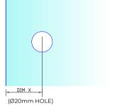
DIM X = 27mm + DIM (t) (GLASS THICKNESS)
