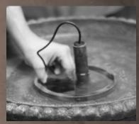
Submerge the water pump in the large bowl and gently shake the water pump under water until there are no air bubbles coming from the vents on the side of the pump.
