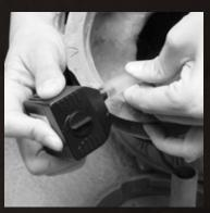
As you can see in the sequence of images above, there is a small length of cord between the water pump and the water seal; giving you enough slack to attach the water pump to the feeder tube inside the fountain bowl while allowing the pump to hang in place, submerged in water when water is added to the fountain.
