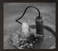
When the pump is running, you should see water flowing from the top of the pump, as shown.
