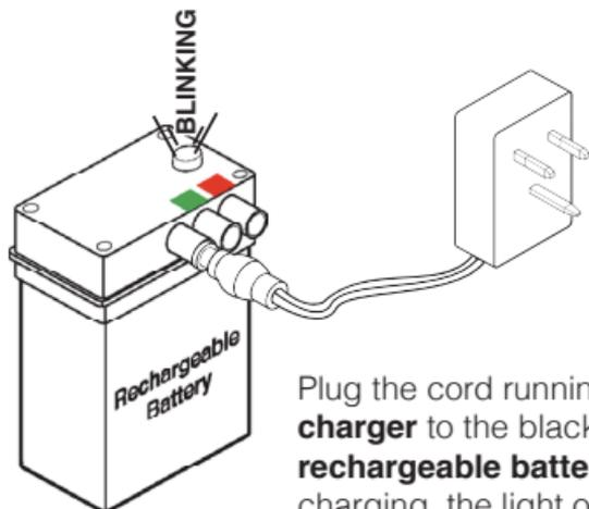
Plug the **battery charger** into an electrical wall outlet.
