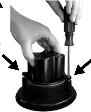
Battery Compartment Retaining Screws X2
