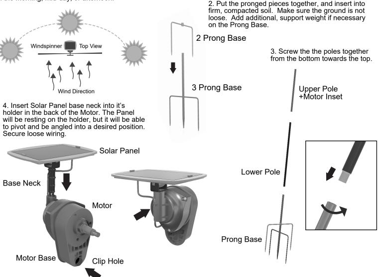
**5.** Insert the Motor Inset inside the Motor Base. Rotate the Motor so the Clip hole at the bottom aligns with the Motor Inset hole. Insert the Motor Clip
