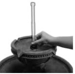
**Step 2:** Attach the extension tube to the water outlet in the middle of the fountain tier. NOTE: Extension must be included.
