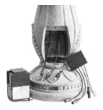
**Step 1:** In the open battery compartment, you will see three cords hanging down that you must connect to the connection port.
