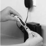
**Step 2:** Take the gray cord that is connected to your battery and plug it into battery charger cord. While the battery is charging, the light on the charger will be solid red.
