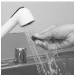
**Step 3:** Wash the filters under running water until debris has been removed. Then replace the filters and pump's front cover.
