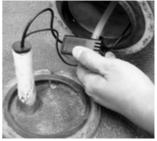
**Step 3:** Reconnect the water pump to the feeder tube inside the fountain tier and reattach the fountain tier to the large bowl.
