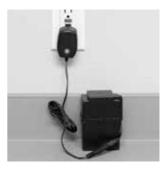
**Step 3:** Charge the battery for 12-14 hours. When the battery is reaching it's fully charged capacity, the light will blink for several minutes. Once the light is a solid green, the battery is at it's full charge. At this point, you can detach the battery from the charger and plug the battery into your fountain.
