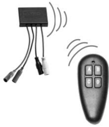
The new wireless remote control (which is not compatible with previous versions of Bernini<sup>™</sup> Fountains) wirelessly connects to the built in receiver inside the connection port.
