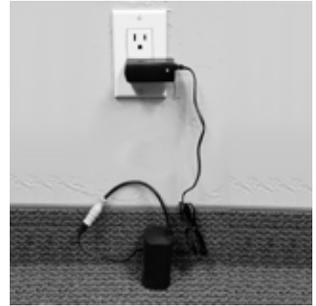
**Step 3:** Charge the battery for 9 hours. When the battery is charging the charger light will be solid red and will turn green when fully charged.
