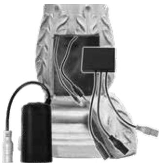
**Step 1:** In the open battery compartment, you will see two cords hanging down that you must connect to the Connection Port.
