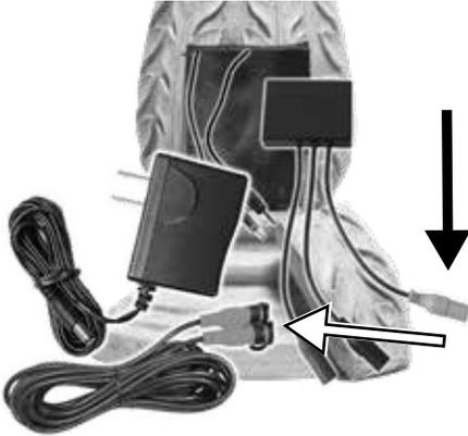
You will be disconnecting the Lithium Battery from the Control Panel and connecting the Extension Cable to the control panel using the same receptacle that the Lithium Battery was connected to (arrows).
