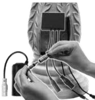
**Step 2:** Using the cords from inside the Base and the cord from the Battery, connect the color coded cords to their corresponding receptacles on the Connection Port.
