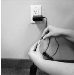
**Step 2:** Take the Yellow cord that is connected to your battery and plug it into battery charger cord. While the battery is charging, the light on the charger will be solid red.
