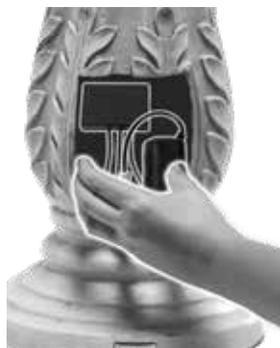
**Step 3:** Place the Connection port into the back of your Base. Then place your Battery inside of the compartment in front of the Connection Port. (See illustration below)
