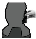
**Step 4:** Place the battery inside of the compartment in front of the connection port. (See illustration 2.1)
