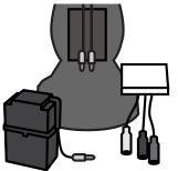
**Step 1:** In the open battery compartment, you will see two cords hanging down that you must connect to the connection port.
