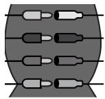
Step 2: Using the cords from inside the base and the cord from the battery, connect the color coded cords to their corresponding receptacles on the connection port.
