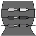
**Step 2:** Using the cords from inside the base and the cord from the battery, connect the color coded cords to their corresponding receptacles on the connection port.
