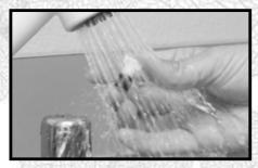
**Step 4:** Rinse the impeller until all debris has been removed. Then replace the impeller in the impeller chamber, put the impeller chamber back on and then replace the pump's front panel.
