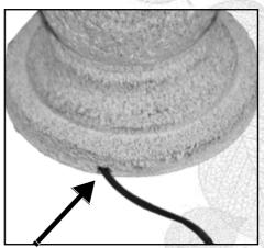
Step 2: Route the Electrical Power Cord through the base of the fountain and through the notch on the bottom of the Pedestal.
