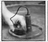
**Step 1:** Submerge the Water Pump(s) into the water inside the Large Bowl and lightly shake the pump underwater to release air bubbles inside the vents on the Water Pump.
