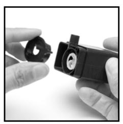
**Step 2:** Remove the impeller chamber cover. This is tightly fitted on to the impeller chamber, but will come off.
