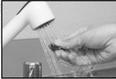
**Step 2:** Wash the filters under running water until debris has been removed. Then replace the filters and pump's front cover.
