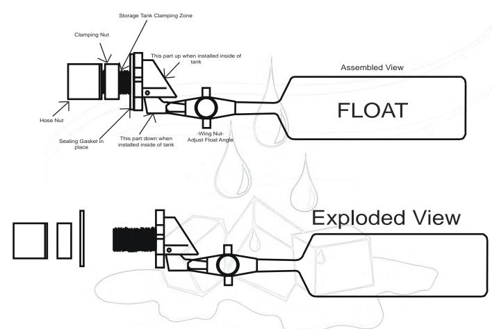
\*\*\*WARNING\*\*\* Improper installation of float valve can and will prevent shut off, causing flooding!!! Monitor installation until you have positive shutoff on system.
