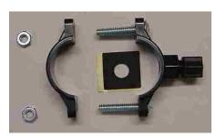
The drain saddle. This drain water is the life blood of the system. If the system cannot drain correctly, it will not function for long. The system is self-flushing and the drain should never be blocked or restricted. This is really simple. The drain saddle is two plastic parts that clamp over the waste water plumbing of your home. There is a small rubber foam washer that needs to be attached to the inside
