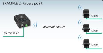
The Wireless Bridge can act as an access point connecting up to seven different slaves. This example shows connection to several Anybus Wireless Bolts. (The Anybus Wireless Bridge and Bolt work seamlessly together.)
