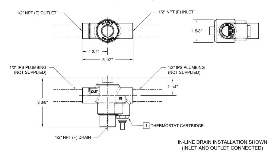
FOR SPECIFIC INSTRUCTION REGARDING INSTALLATION, RETRO-FIT, MAINTENANCE OF THIS MODEL CONTACT HAWS TECHNICAL SUPPORT AT 1-800-766-5612.
