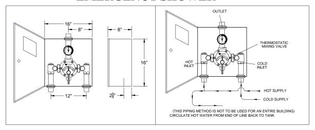
CAUTION! It may be necessary to recirculate the tempered water to the emergency shower should the piping be exposed to excessive hot or cold conditions. Consult factory for proper piping.
