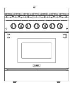
LP: Input Pressure: 11 inches Output Pressure: 10 inches Regulator Location: Inside the kick Panel – Bottom Right Size of Regulator: ½ inch
