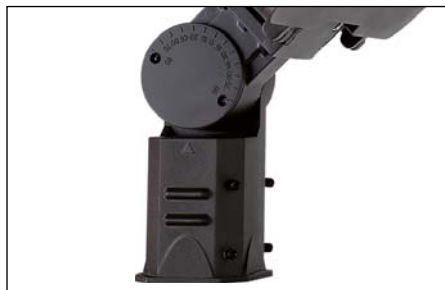
Slipfitter Mount An optional cast aluminum mast arm adapter secures fixture head to nominal 2"(2-3/8" O.D. pipe size) horizontal steel tenon arm.
