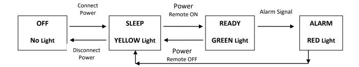
Note: When the system is in Remote Only (RO) mode, only the Remote can be used to go between the SLEEP and READY states or to switch the alarm OFF. The Power button will not function. This will be explained later.
