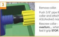
Remove collar. Push 3/8" pipe through collar and attach to AQUAvalve5 nozzle. Rescrew collar - DON'T overturn... when you
