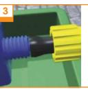
Remove collar. Push 3/8" pipe through collar and attach to AQUAvalve5 nozzle. Rescrew collar - DON'T overturn... when you
