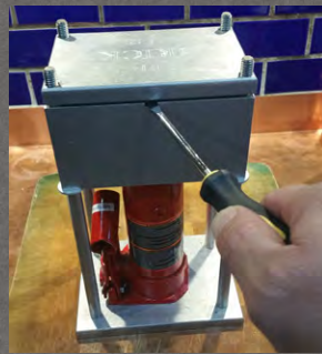
FIGURE 15 Remove the wing nuts. Using a flathead screw driver, USE the notch behind the Press body to help unseal the lid from the Press body.
