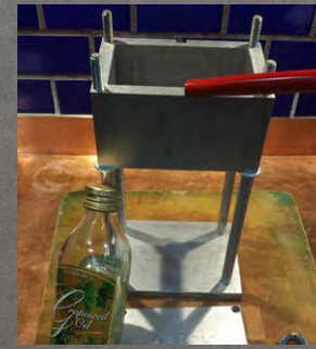
FIGURE 5 Lightly lubricate the top rim of the Press body with a light film of Grapeseed oil.
