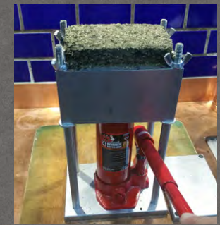
FIGURE 18 Place the handle back into the jack and begin pumping the newly pressed material out the top along with the plug.
