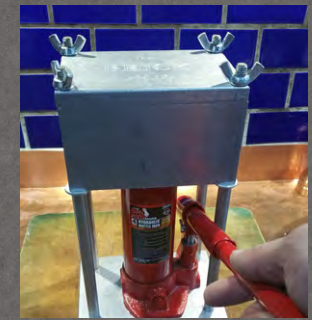
FIGURE 12 Begin pumping the jack handle until you can no longer pump it by hand. DO NOT try to apply any additional force once the plug has bottomed out under normal hand pumping.
