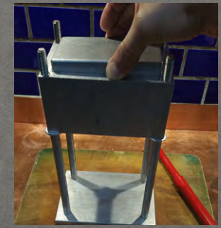
FIGURE 6 Gently place the plug back inside the Press body making sure that it goes in straight and not at an angle.
