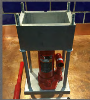
FIGURE 9 The Press is now ready to begin filling.
