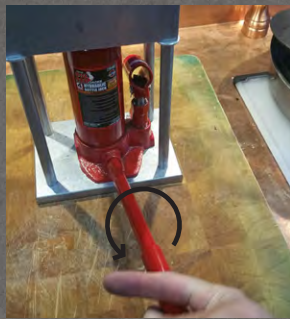
FIGURE 14 When cool, place the Press right side up and turn the valve counter clockwise to relieve the pressure.
