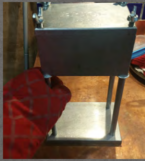
FIGURE 2 After 5 minutes of boiling, remove the Press from water using oven mitts. Metal will be very hot.
