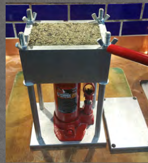
FIGURE 16 Once the lid is removed, Replace all 4 wingnuts back on to the Press body.
