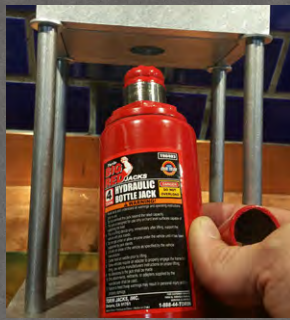
FIGURE 8 Place the jack underneath the plug making sure that the piston seats into the port. IMPORTANT! Failure to properly center the jack will cause the plug to rise crookedly and jam.
