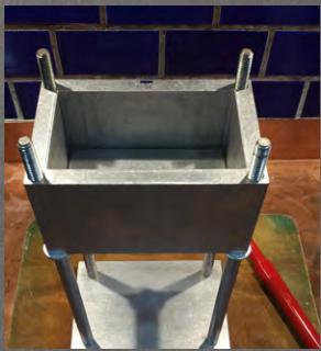
FIGURE 7 Make sure that the plug is in its furthest downward position and resting on the washers/ledge below.
