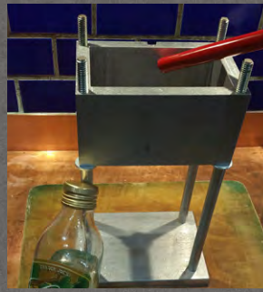
FIGURE 3 Remove the wing nuts, lid and brick from the Press body. Using Grapeseed oil, lightly lubricate inside the Press body.
