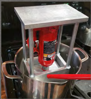
FIGURE 13 Allow the Press to cool before attempting to open. The material MUST remain under pressure while cooling. To expedite the cooling process, you may place the Press upside down in a pot of ice water for 1 hour.
