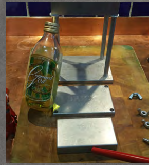
FIGURE 4 Lightly lubricate all surfaces of plug with a light film of Grapeseed oil.
