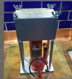
FIGURE 11 Place the lid onto the Press body, tighten the wing nuts and turn the valve on the jack clockwise.
