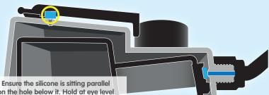
on the hole below it. Hold at eve level to check the position is correct
